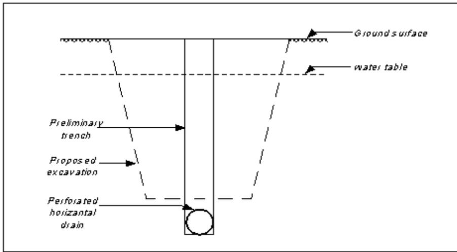
**Figure 3: Horizontal Drainage System (After Johnson, 1972)**
