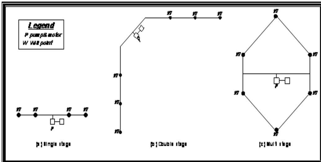
**Figure 4: General Forms of Well Point System (after Johnson, 1972)**
